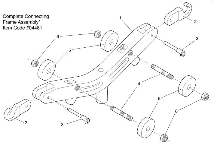
\*Connecting Frame Assembly #04481 does not include part #2 (Chain Hook) & part #3 (Release Pin). These items must be ordered separately. Please refer to chart below.
