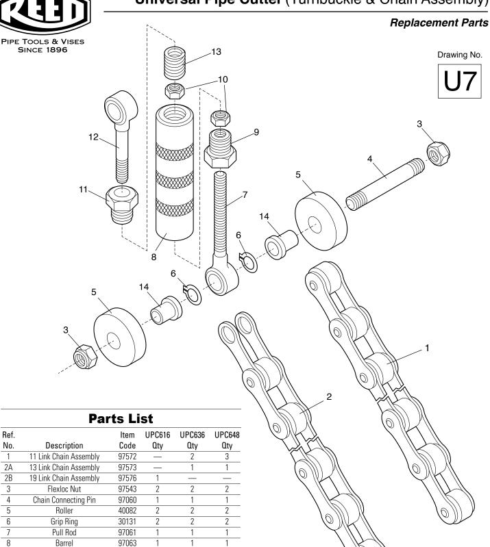
Complete Turnbuckle & Chain Assembly #97579 UPC636, UPC648 #97580 UPC616 (Item #1 not included with either)
